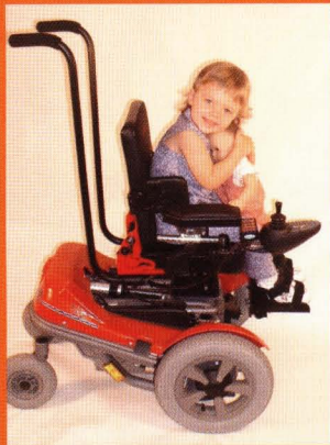
TheBUG OiS – Shown here with an Oxygen Cylinder adapter on the back of the frame. The cylinder articulates as the upper assembly is tilted.
